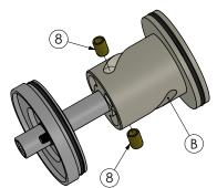
8. Remove the piston (10) from the baseplate assembly (27).
