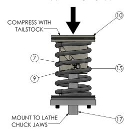
8. Remove the retaining ring (9) and press the axle (7) through the shaft's axle bore (A) and piston's helical track (B).
