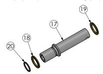
4. Insert the shaft (17) into the base plate (22).
