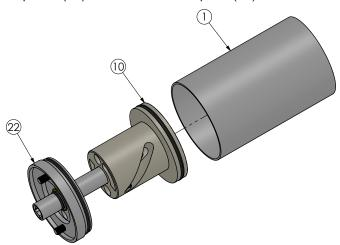
10. Insert the guide bars (2,3) into the bores on top of the piston (10) and align them with the bores in the base plate (22).
