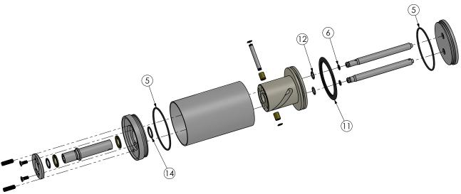
2. Thoroughly grease the inside of the casing (1) and piston (10).
