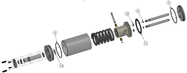
2. Thoroughly grease the inside of the casing (1) and piston (10).
