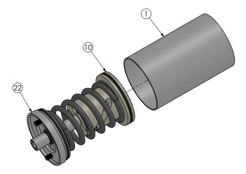
13. Insert the guide bars (2,3) into the bores on top of the piston (10) and align them with the bores in the base plate (22).
