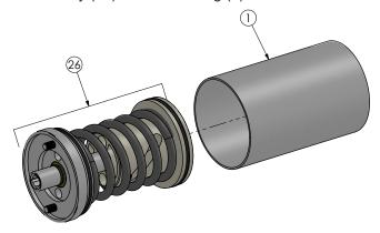
7. To remove the piston (10) from the assembly, we recommend using a lathe. Mount the shaft (17) on the lathe using soft chuck jaws and press the tailstock against the top of the piston (10). Compress the spring (15) with the tailstock enough to provide access to one of the axle (7) retaining rings (9).
