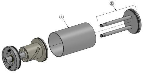
5. Remove the base plate/piston assembly (26) from the casing (1).
