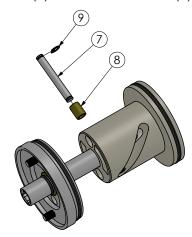
7. Insert axle (7), with track roller (8) installed, into helical slot (B) and through axle bore (A).
