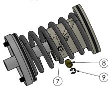
11. Relieve the springs tension by backing off the tailstock completely and remove the base plate/piston assembly from the chuck jaws.
