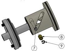
9. Slide the casing (1) over the piston (10) and onto the base plate (22).
