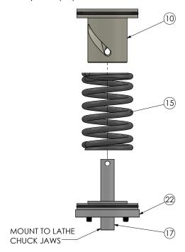
7. Compress the spring (15) with the tailstock until the shaft (17) is inserted into the bore of the piston (10). Continue tensioning the spring until the shaft's axle bore (A) is aligned with the helical track (B) and is accessible for the installation of the axle assembly.
