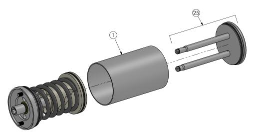
6. Remove the base plate/piston assembly (26) from the casing (1).
