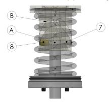
10. Slide the second track roller (8) onto the axle (7) and mount the second retaining ring (9).
