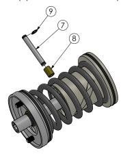
9. Insert axle (7), with track roller (8) installed, into helical slot (B) and through axle bore (A).
