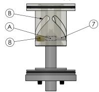
8. Slide the second track roller (8) onto the axle (7) and mount the second retaining ring (9).
