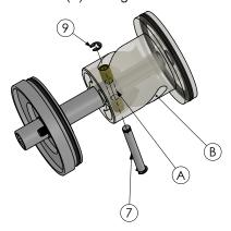
7. Remove the track rollers (8) from the piston's helical track (B).
