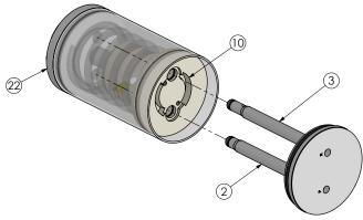
14. Insert the flange (16) into the bottom of the base plate (22) and align the counter sunk holes with the bores in the base plate (22). While pressing down on the top plate (13) install and firmly tighten the flat head screws (4).
