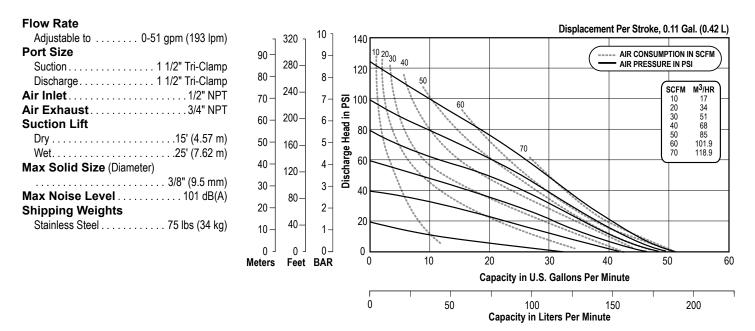
NOTE: Performance based on the following: PTFE fitted pump, flooded suction, water at ambient conditions. The use of other materials and varying hydraulic conditions may result in deviations in excess of 5%.
