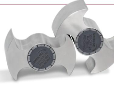
All-metal rotors offer an alternative approach that eliminates the risks associated with plastic. Unibloc CleanPlus rotors are milled from a single billet of stainless-steel, avoiding weld transitions that could harbor product or bacteria.
