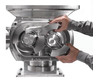
This common approach to securing the rotors creates a delicate balance. Maintenance technicians must torque bolts carefully to specification: excessive torque can crush sleeves or cause shaft deflection, leading to leaks and housing damage, while insufficient torque risks bolts backing out during operation. Unfortunately, technicians are
