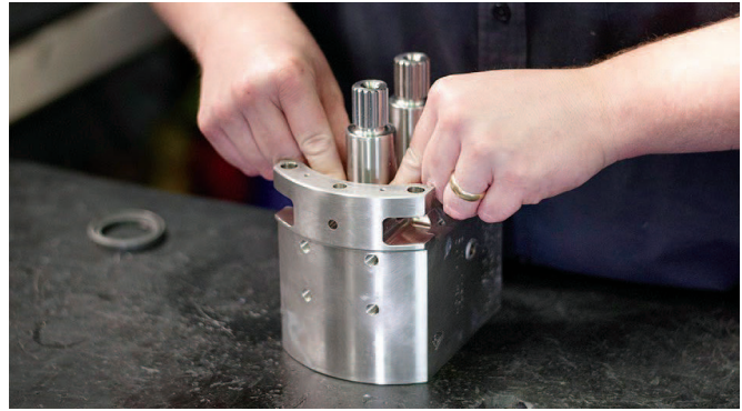
A gear pump with a clean or simplified design makes maintenance much easier for sanitary operations.
