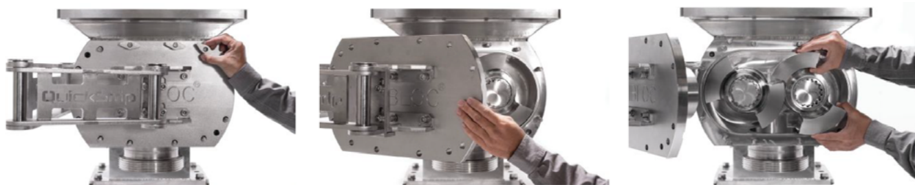
An example of a COP pump design from Unibloc Pump. Without tools, cleaning crews can quickly open the pump cover, swing it aside and remove the pump rotors.
