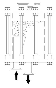
Standard configuration shown. Standard 316L, 20 Ra and electropolished. Other finishes and port configurations are available.
